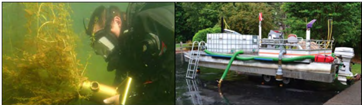
Figure 64: DASH – Feeding EWM into the underwater Suction Hose (Marinette Co.); and a sample DASH Pontoon Boat (Beaver Dam Lake Management District)
