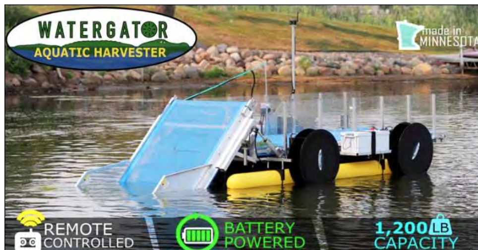
Figure 66: WaterGator remote-controlled aquatic plant harvester (https://lakeweedharvester.com/watergator/)
